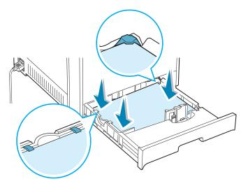
**5** Do not exceed the maximum stack height. Overfilling the tray may cause a paper jam.
